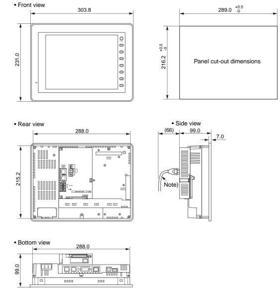
2-2-2 External dimensions and panel cut-out dimensions for the NP5M0101-4H4/NP5N0011-4H4 (Unit: mm)
